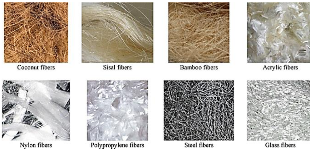
Figure 3: Various fibre additives used in concrete, including natural, synthetic, and steel fibres [16]
