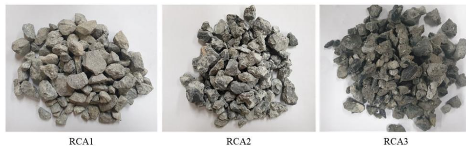
Figure 2: Recycled concrete aggregates with different recycling generation. [1]
