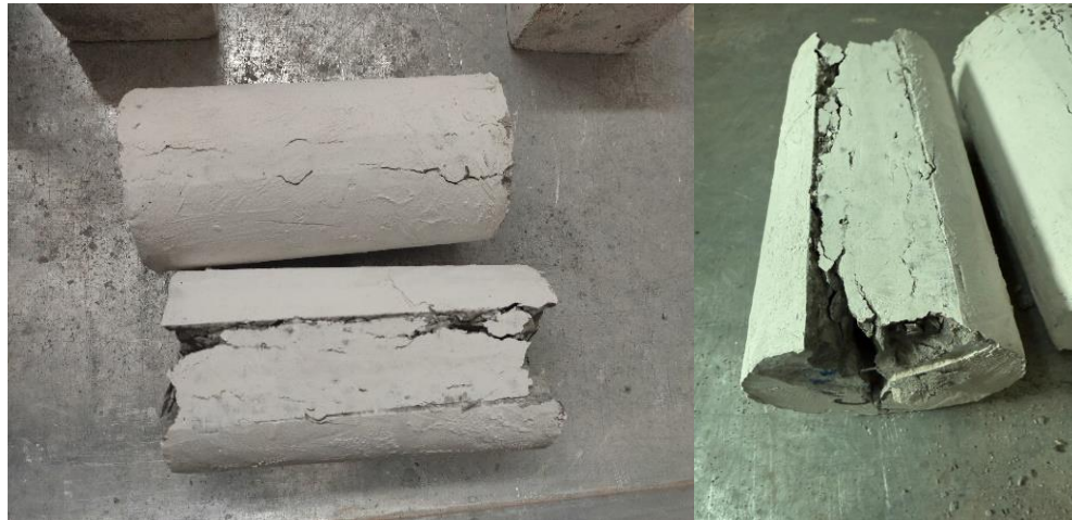
Figure 1: Tested specimen under splitting tensile load
