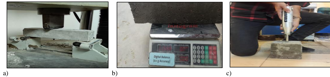
Figure 3: a) Beam under flexural load test, b) water absorption test c) Schmidt hammer test
