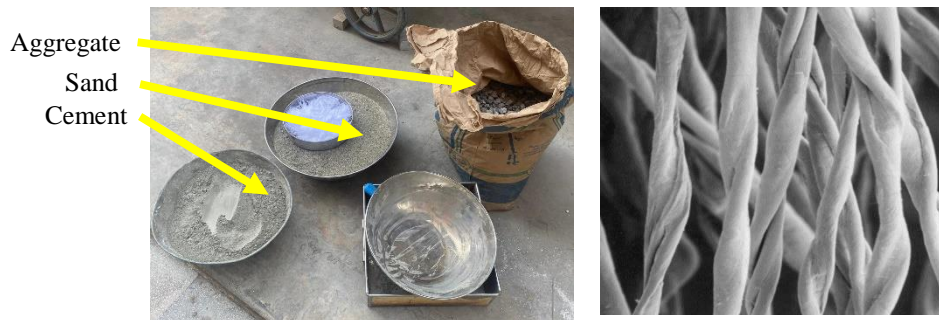
Figure 1: Raw materials used for samples preparation (Left) and microscopic view of Cotton Fibre Thread (Right)
