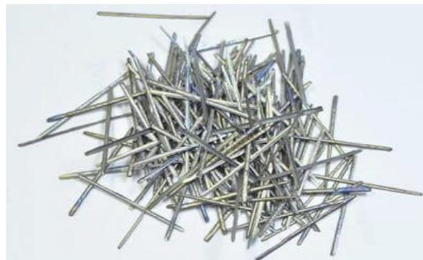
Figure 2: Steel Fibers in concrete matrix [31]
