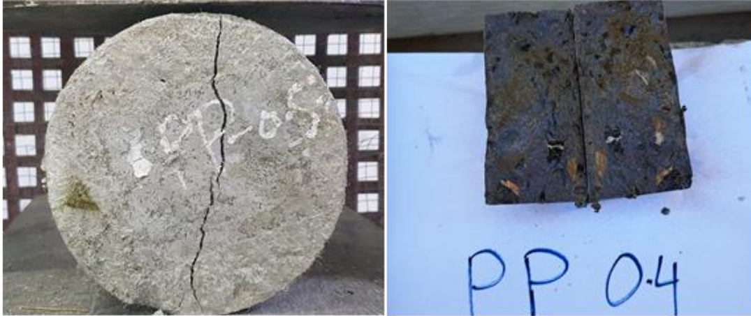
Figure 4: Split tensile strength test of cores taken from prestressed beams
