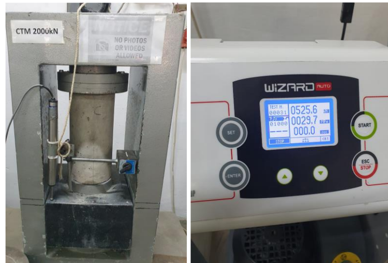
Figure 3: standard cylinders in the compression testing machine (CTM) having 2000 KN capacity
