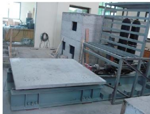
Figure 8. Shake table at UET Peshawar
