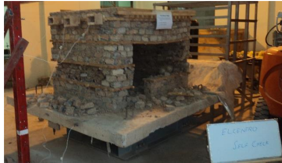
Figure 13. Damages at the end of the test
