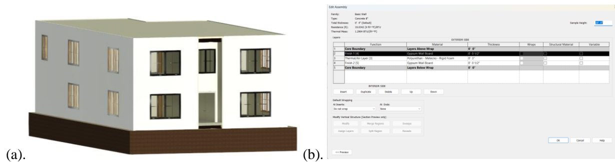
Figure 2 BIM based Revit Model of NIEC lab building: (a). Full architectural model representing actual site layout (b). Wall material properties defined for simulation
