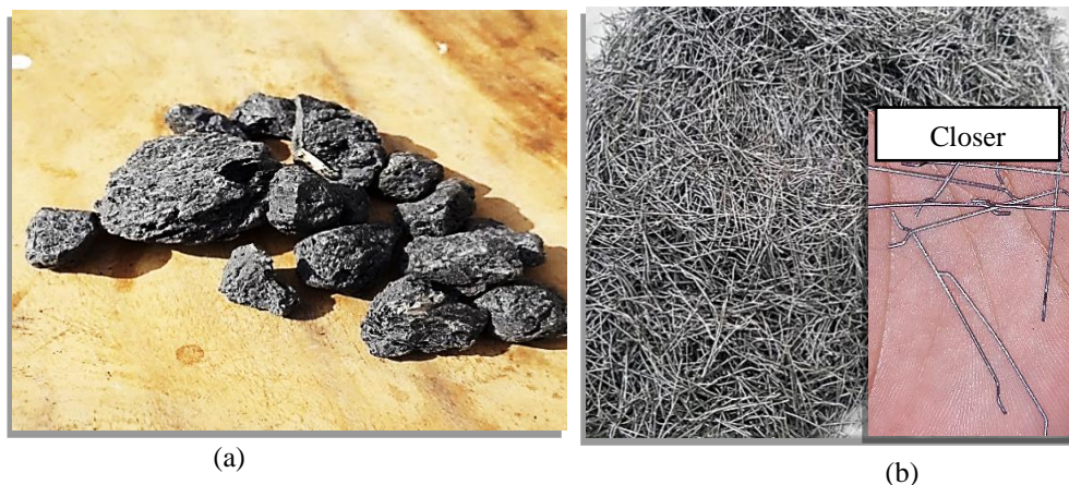
Figure 2: (a) The prepared E-waste aggregates and (b) the used Steel fibres
