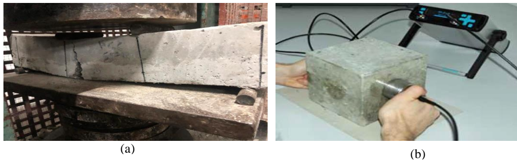
Figure 5: (a) flexural strength testing and (b) UPV testing
