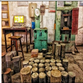
Figure 3: Lab testing, a. Cylinders under process in compression testing machine after fire, and b. Compression test results
