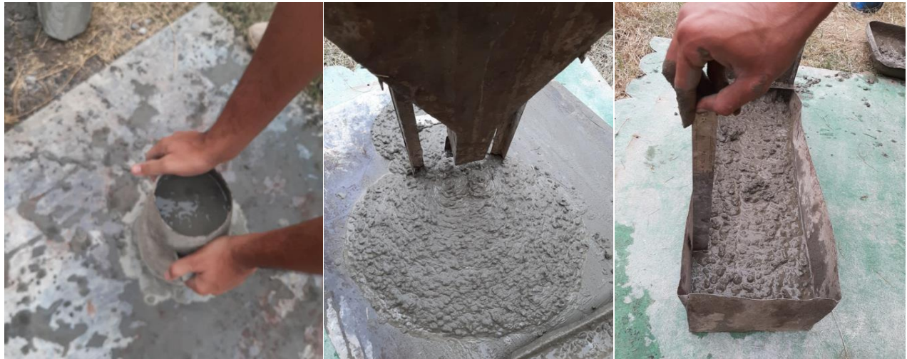
Figure 1: Evaluating Fresh properties of developed SCC.
