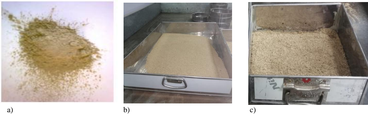
Figure 1: a. Dust remove from the rice husk, b. small particles, c. selected rice husk particles for test
