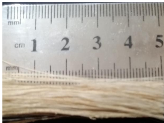
Figure 1: Combed banana fibers of 50mm length.
