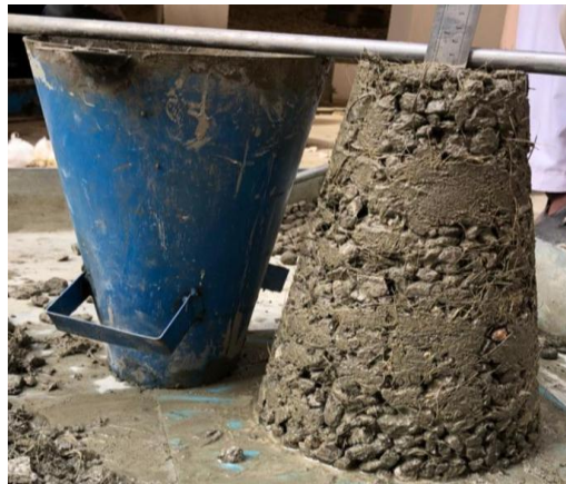
Figure 2: Measuring the slump value of BFRC
