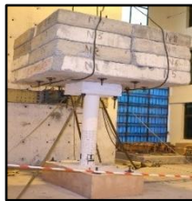
Figure 2. Test assembly setup with physical loading of 42.4 Kips.
