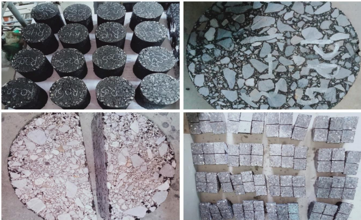
Figure 3: Preparation of Semi Circular Shaped SCB Test Samples from Gyratory Samples
