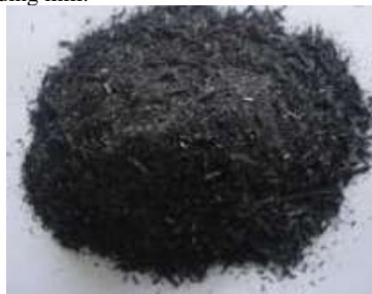
Figure 3: Wheat Straw Ash at 600 °C
