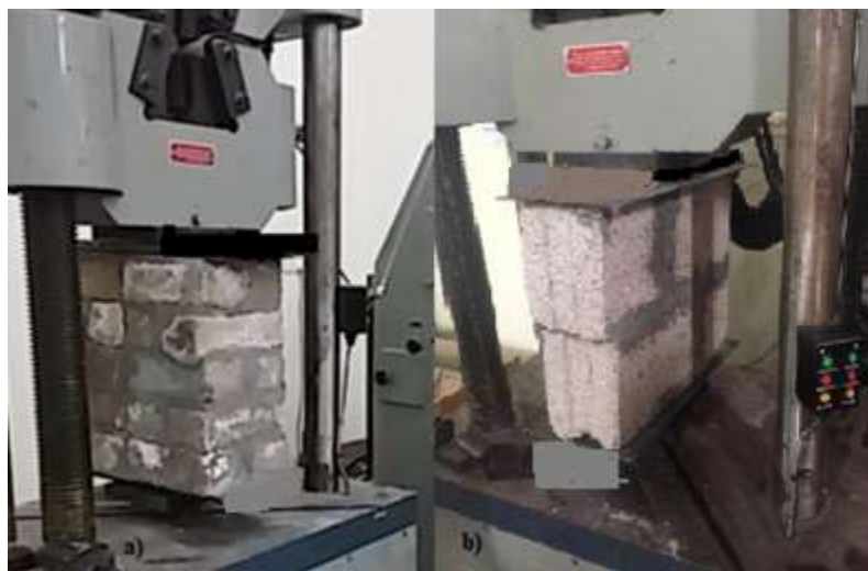
Figure 1: Testing of Masonry Prisms
