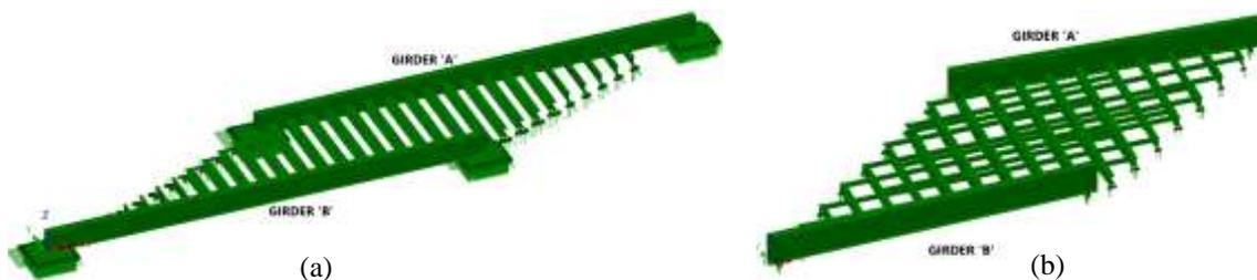
Figure 2: (a) Grand Union Canal LUSAS Shell Model; (b) Battersby Lane LUSAS Shell Model. Floor deck excluded for clarity
