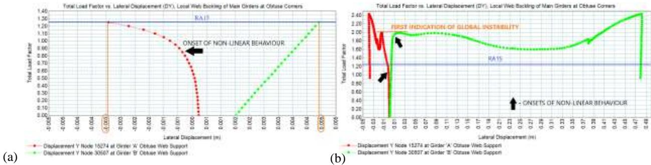
Figure 4: (a) Non-linear buckling analysis 1, last load increment at factor 1.25 x RA1 live load; (b) Non-linear buckling analysis 2, highest load increment peaks at ~2.4 x RA1 live load.
