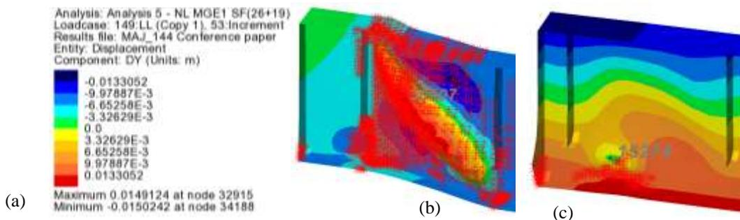
Figure 5: Displacement contours at buckled panels at load increment 2.0 x RA10 railway live load (non-amplified). Red crosses indicate yielded mesh. (a) Contour legend; (b) Node 30507, buckling at obtuse end of Girder 'B', signifying tension field action; (c) Node 15274, localised buckling at obtuse end of Girder 'A'.
