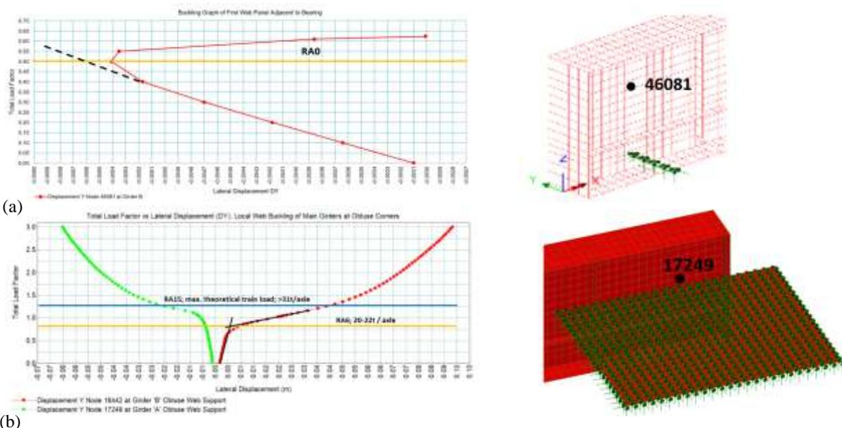
Figure 3: Web buckling behaviour at obtuse corners of the girders. (a) Simple support conditions; (b) Slideline surfaces.
