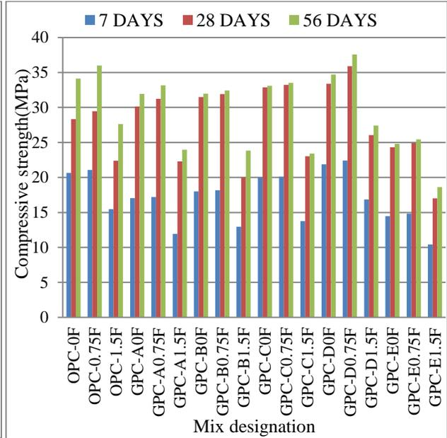
Figure 3: The result of compressive tests of the mixes
