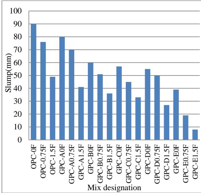
Figure 2: The result of slump test of the mixes
