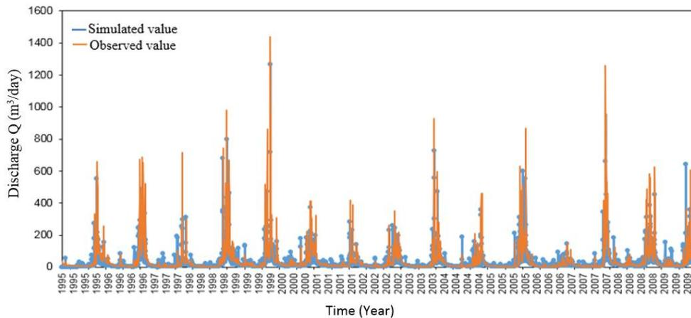
Figure 4: Calibrated (1995-2002), and validated (2003-2009) hydrographs of discharge at An Lao station
