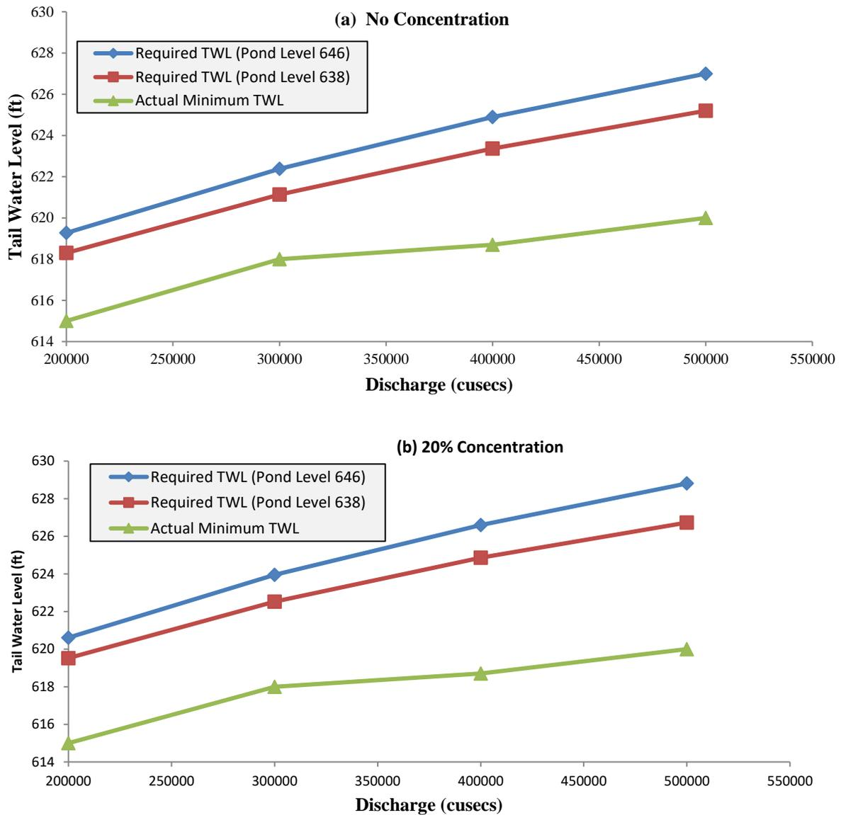
Figure 4: Comparison of Required and Existing Tail Water Levels (TWL) for various Discharges Passed at Different Pond Levels
