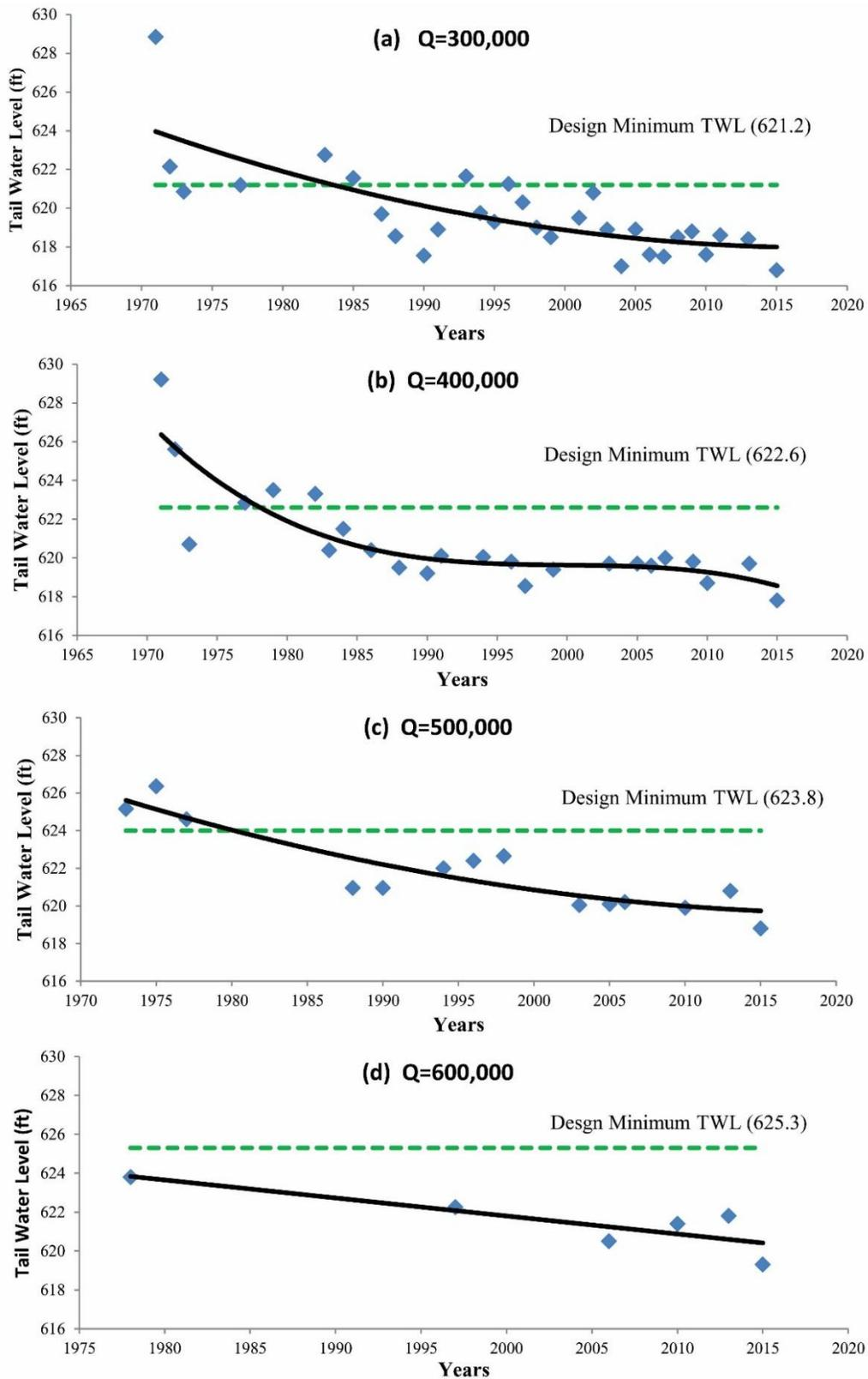
Figure 3: (a,b,c&d) Degradation Trends of Tail Water Levels at various Discharges
