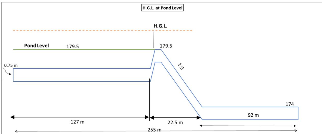
Figure 3: Cross-sectional view of Chiniot barrage
