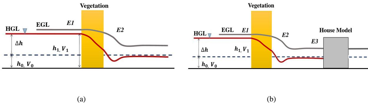
Figure 4: Flow behavior and difference of different parameters in the presence of (a) only vegetation and (b) vegetation with a house model.
