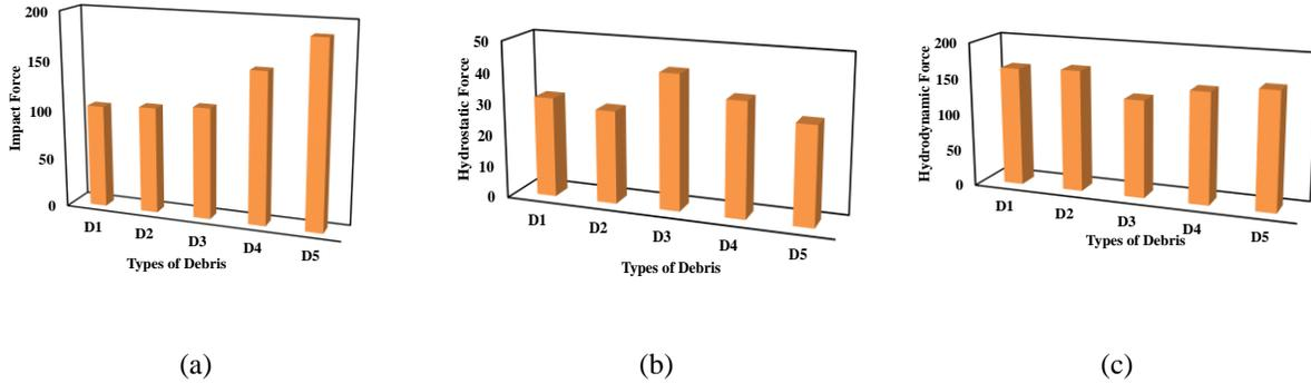
Figure 2: Comparison of waterborne debris (a) impact force (b) Hydrostatic force (c) Hydrodynamic force
