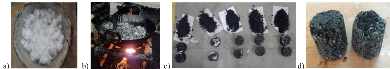
Figure 1: a. Polypropylene fibers before addition. b. Polypropylene-fiber modified sample being prepared. c. Compacted and loose samples ready for Marshall stability test. d. Polypropylene-fiber modified samples after Stability test
