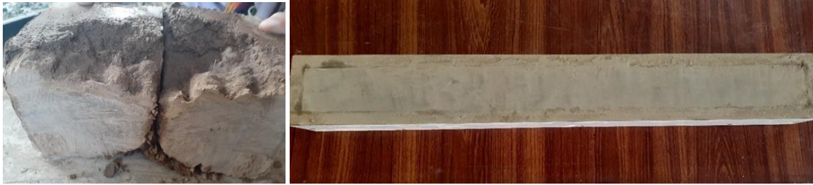
Figure 2a: Post-test condition of specimens, a. after spray erosion test, and b. linear shrinkage box test
