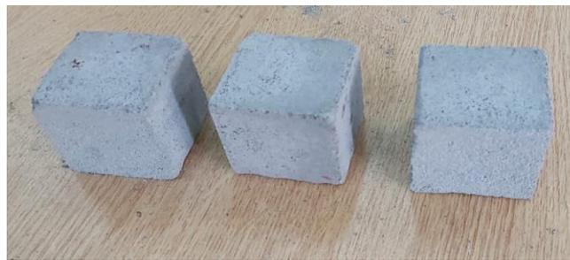
*Figure 4: WPSA (25%) Mortar Samples.*
