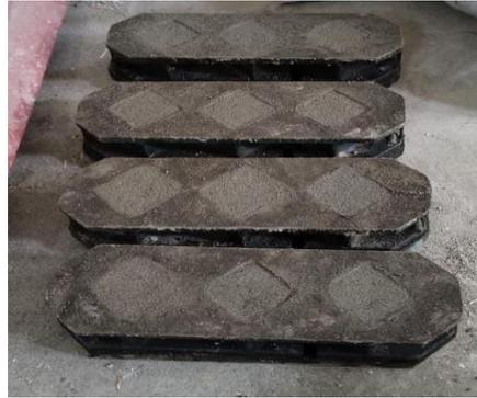
*Figure 3: Mortar mix Casted in Moulds.*
