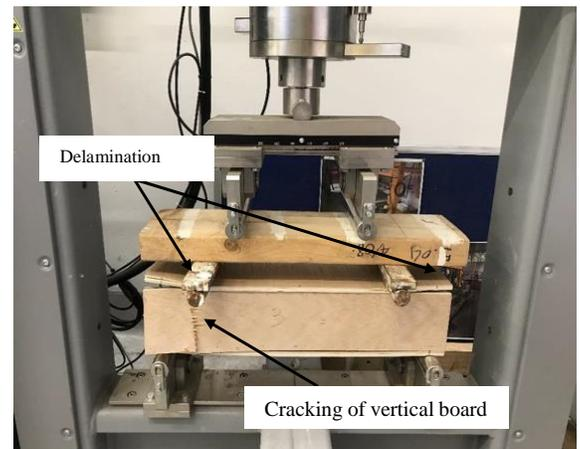
Figure 4: Failure mode of beam
