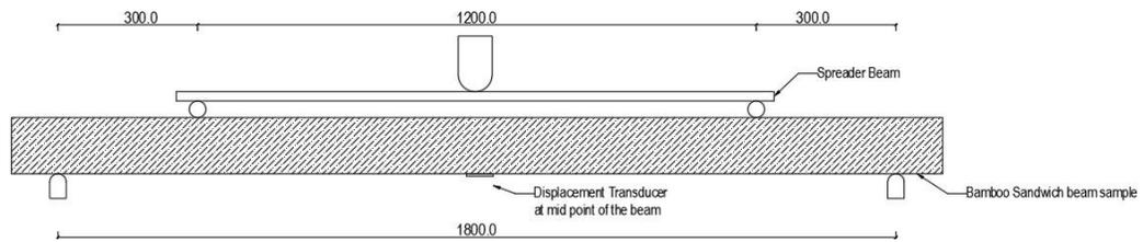
Figure 2: Test setup for four-point loading on 2m beam
