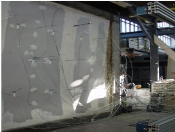
a) Bowing in test wall (one hour exposure)
