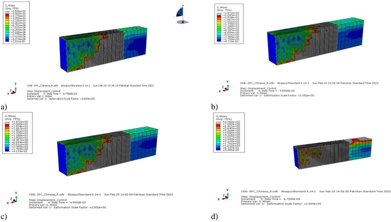
Figure 3: a. Retrofitted GPC Beam stresses, b. 0.75SF-GPC Retrofitted Beam Stresses, c. 0.5SF+1SsF-Retrofitted-GPC Stresses, d. 2.4SsF-Retrofitted-GPC beam Stresses
