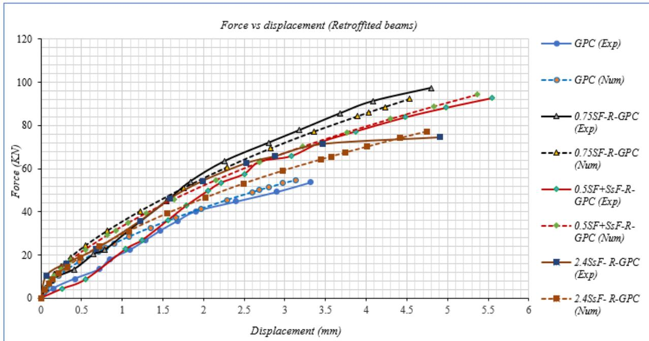
Figure 4: Load Vs Displacement (Controlled & Retrofitted Beams)
