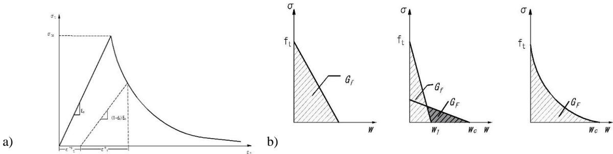
Figure 4: a. Typical uniaxial tensile stress-strain curve and, b. linear, bi-linear and exponential relations for tension stiffening.
