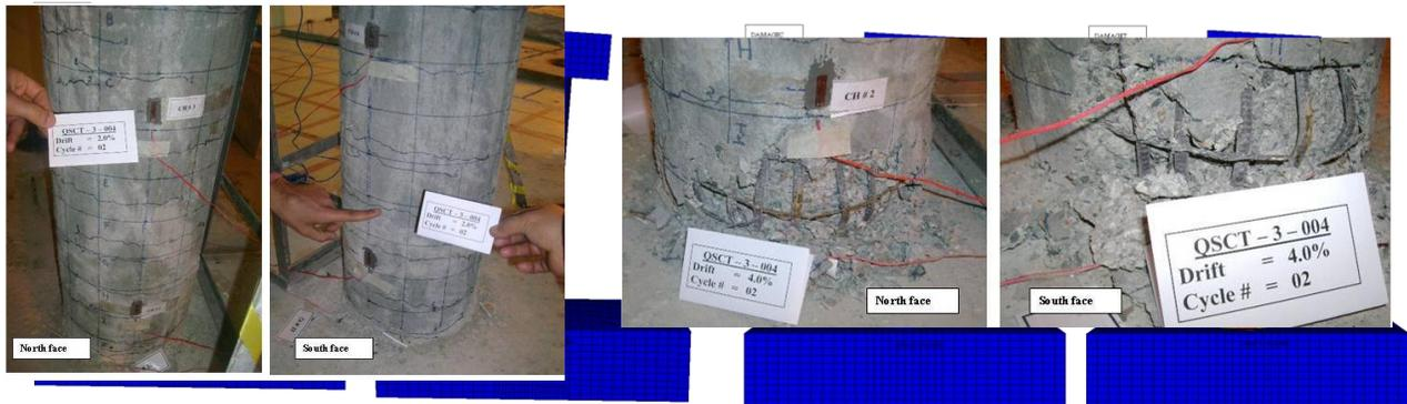
Figure 8: Failures observed in the experimental test a) Tensile cracking, b) Compressive crushing of concrete and rebar yielding
