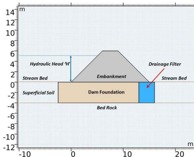
Figure 1: Cross-section of the dam and boundary conditions
