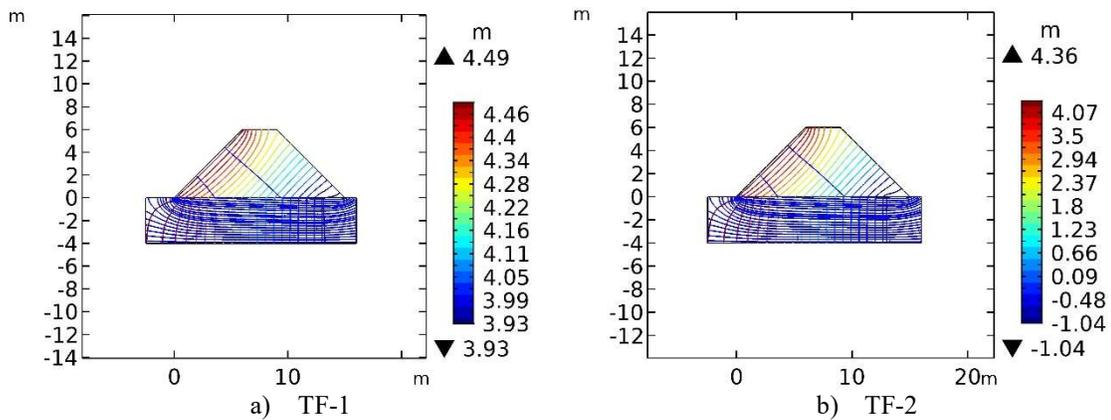
Figure 2: Flow net patterns with different filters, the legend shows the hydraulic head.
