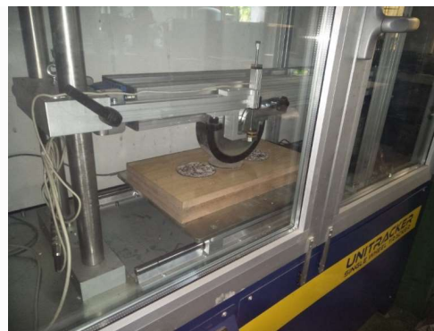
Figure 6: Wheel Tracker Test
