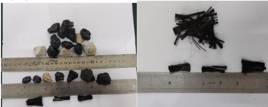
Figure 2: Manufactured Plastic Aggregates and Carbon Fibres
