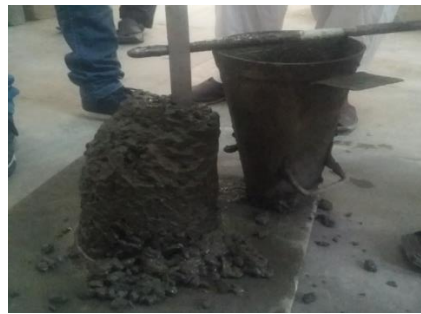
Figure 5 Slump Cone Test
