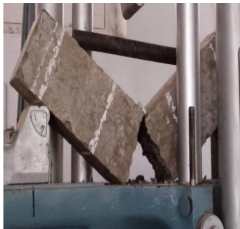
Figure 11 Prismatic Specimen after Testing
