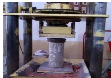
Figure 7 Cylindrical Specimen during Testing
