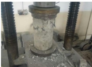
Figure 6 Compressive Strength Setup
