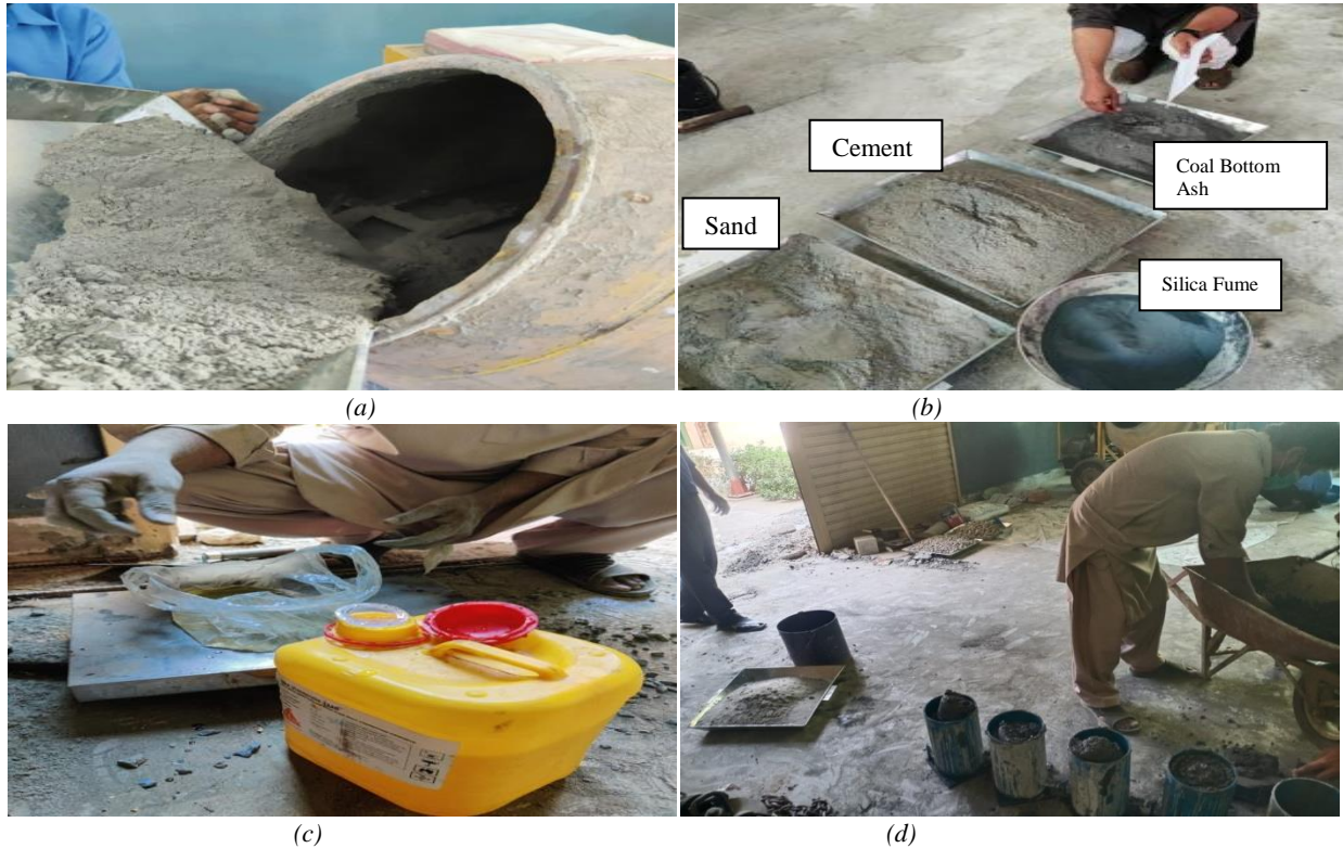
Fig.2: Preparation of samples, (a) Dry mixing of ingredients, (b) CBA, FA & OPC, (c) Super plasticizer (SP) Viscocrete-3110, (d) freshly casted cylinders
