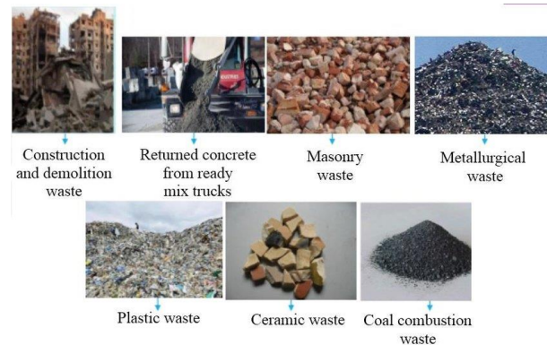
Figure 3 Different types of Recycled Aggregates (Makul et al., [37])
