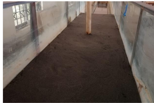
Figure 2b: Compound pier with levelled bed
