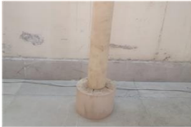
Figure 2a: Photograph showing the model of compound circular bridge pier used in the current study
