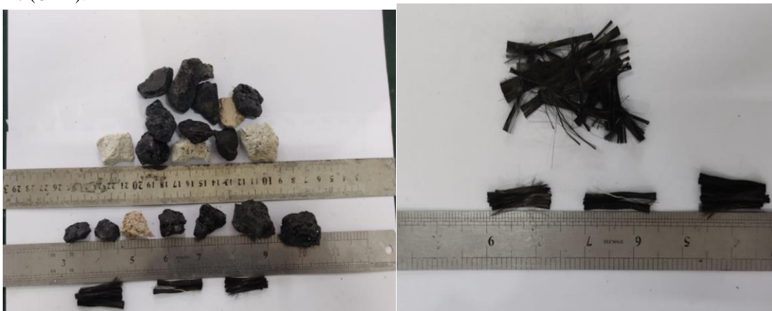
Figure 2: Manufactured Plastic Aggregates and Carbon Fibres
