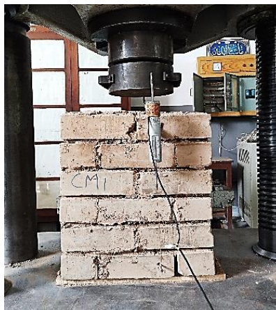
Figure 2 Experimental setup for masonry compressive strength
