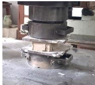
Figure 1 Experimental setup for CSEB unit compressive strength
