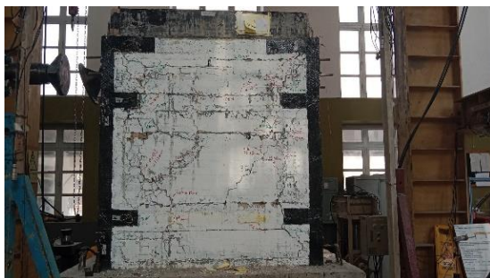
Figure 3: Retrofitted CM results, a. Failure of retrofitted confined tie column b. Envelope curve
