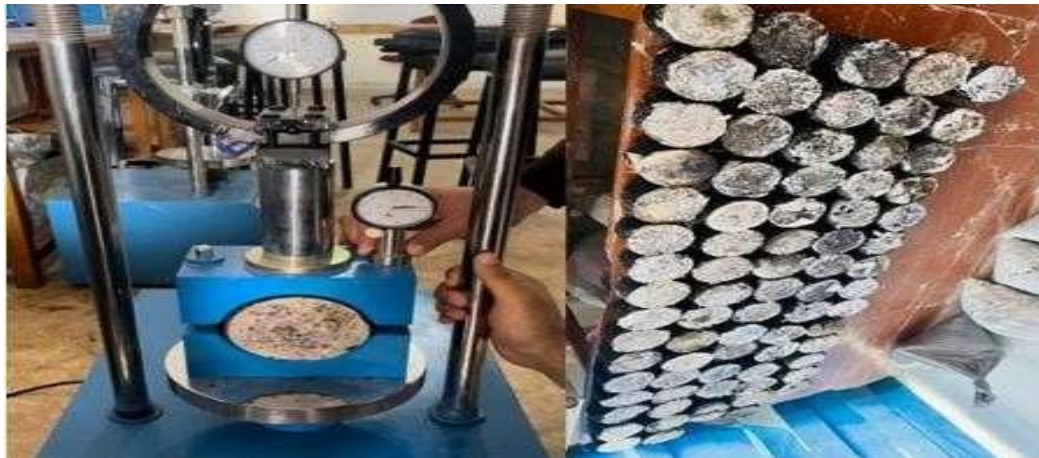
Figure 1: Marshall Apparatus and Marshall Molds
