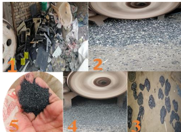
Figure 3 Detail process of preparation of PFA
