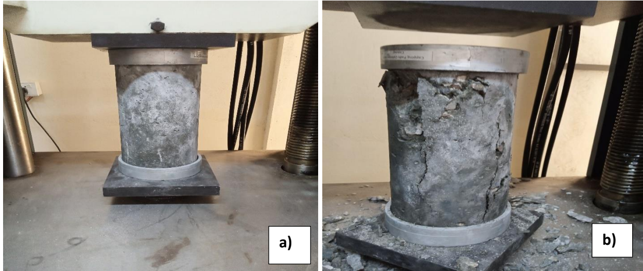
Figure 3: Compression test Assembly a. Cylinder before test and b. Cylinder After test
