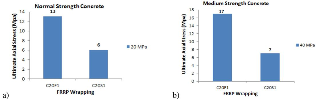
Figure 10: Effect of FRRP Spacing on ultimate axial stress, a. normal strength concrete, and b. medium strength concrete
