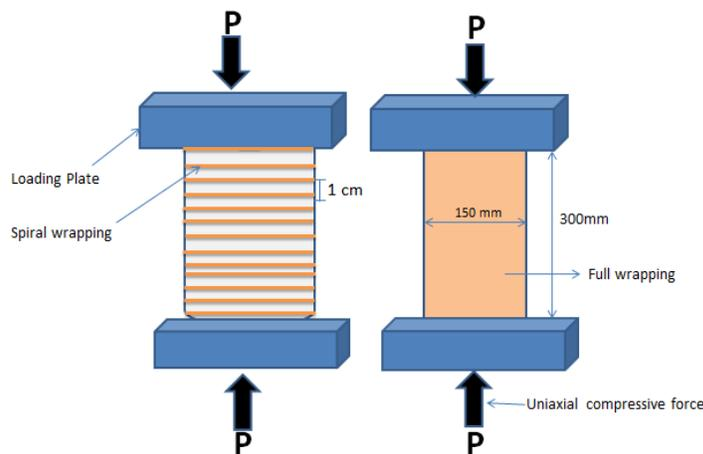
Figure 1: Schematic diagram of concrete specimens showing spiral and full FRRP wrapping
