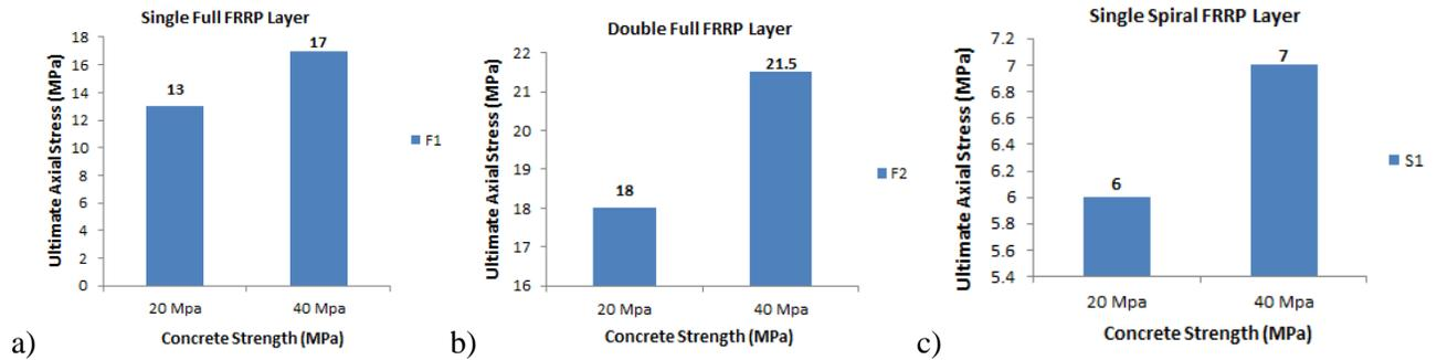
Figure 7: Effect of concrete strength on ultimate axial stress, a. single layer of FRRP, b. double layer of FRRP, and c. spiral layer
