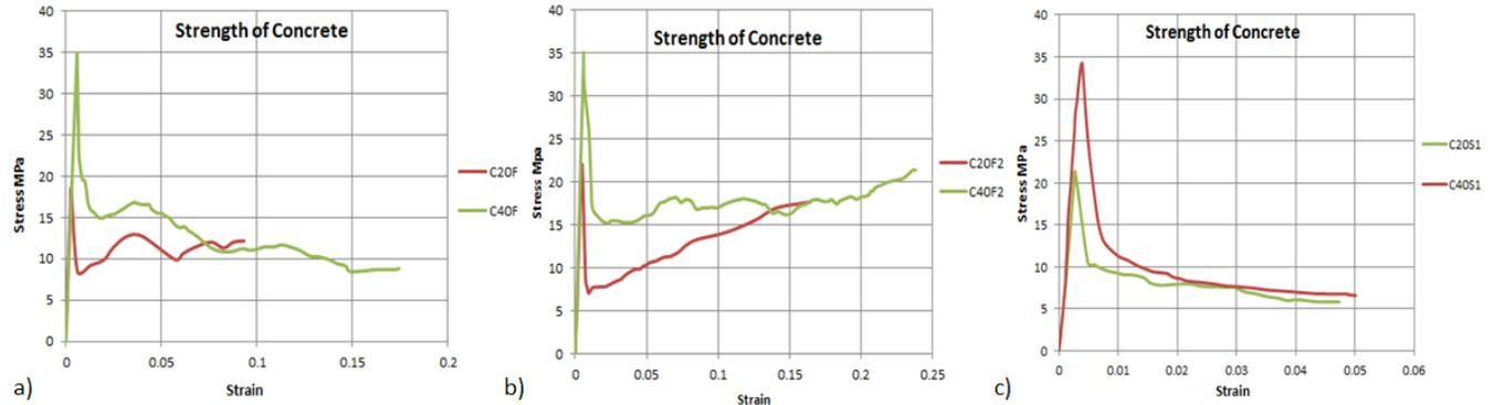
Figure 6: Effect of concrete strength on stress-strain response, a. single layer of FRRP, b. double layer of FRRP, and c. spiral layer
