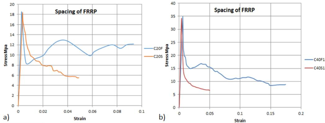
Figure 9: Effect of FRRP Spacing on stress-strain response, a. normal strength concrete, and b. medium strength concrete
