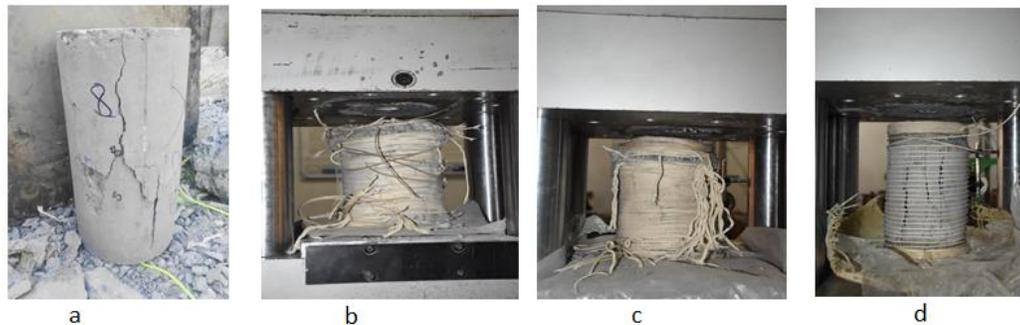
Figure 13: Typical failure modes of 40 MPa FRRP specimens, a. control, b. full single layer, c. full double layers, and d. spiral layer.
