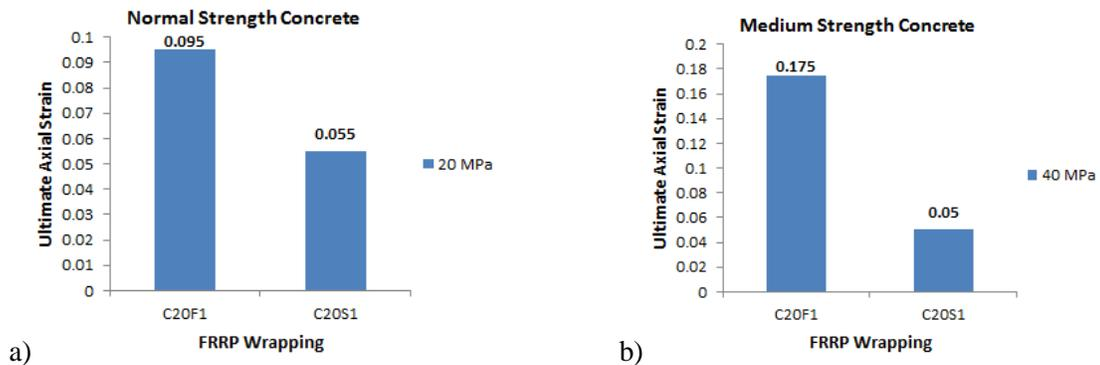
Figure 11: Effect of FRRP Spacing on ultimate axial strain, a. normal strength concrete, and b. medium strength concrete
