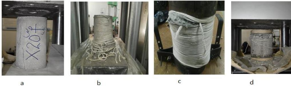
Figure 12: Typical failure modes of 20 MPa FRRP specimens, a. control specimen, b. full single layer, and c. full double layers and d) spiral layer.
