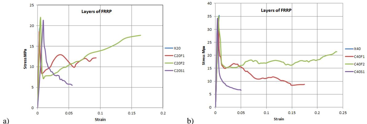
Figure 3: Effect of FRRP layers on stress-strain response, a. normal strength concrete, 20MPa, and b. medium strength concrete, 40MPa
