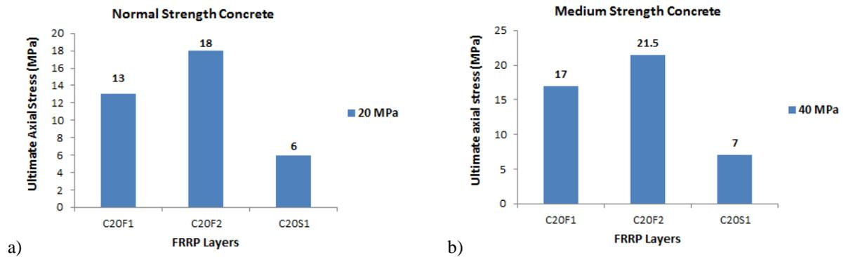
Figure 4: Effect of FRRP layers on ultimate axial stress, a. normal strength concrete, and b. medium strength concrete
