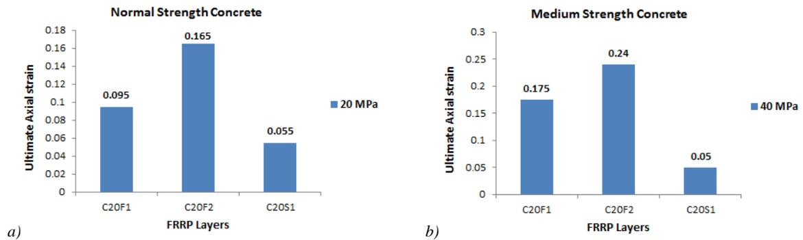
Figure 5: Effect of FRRP layers on ultimate axial strain, a. normal strength concrete, and b. medium strength concrete
