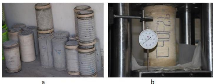
Figure 2: Specimens wrapping and instrumentation details, a. cotton FRRP wrapped specimens, and b. instrumentation and loading setup
