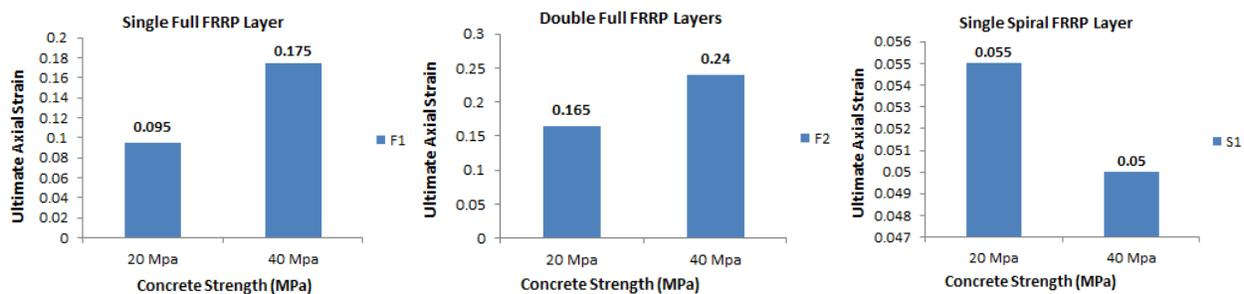
Figure 8: Effect of concrete strength on ultimate axial strain, a. single layer of FRRP, b. double layer of FRRP, and c. spiral layer
