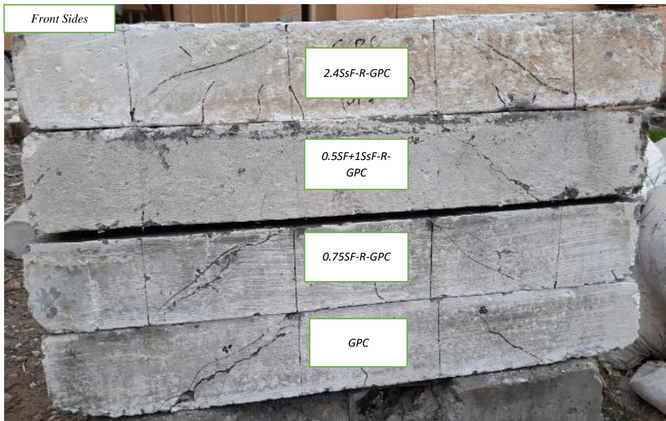
Figure 2: Shear failure of the beams
