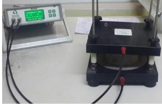
Figure 2: Concrete resistivity meter (AC) and testing of the specimen
