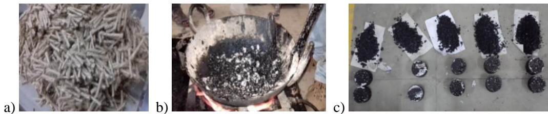
Figure 1: a. Jute fibers before addition. b. Jute-fiber modified sample being prepared. c. Compacted and loose samples ready for Marshall stability test
