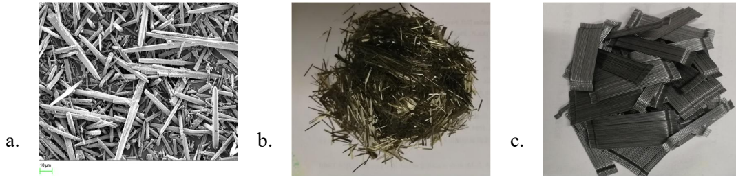
Figure 1: Raw materials, a. CaCO 3 whiskers, b. basalt fibers, and c. steel fibers
