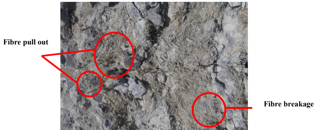
Figure 4: Fibre behavior in broken test specimen
